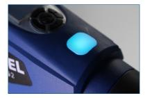
The upload progress is shown on the display. As long as the upload is active, the control LED lights up **BLUE**.
